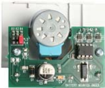
Electronic Drive Motor with Selectable rotational Speeds
