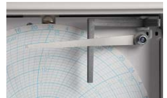
Pen arm lifter, which allows the pen to be raised whilst changing charts.
